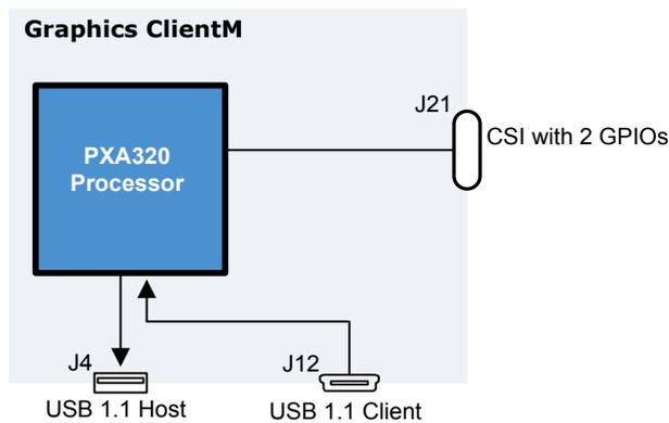
The third option provides two USB 1.1 host ports on socket J4 (dual socket option) and a CSI on socket J21. The CSI uses ten of the twelve GPIOs. In this option, socket J12 is not populated, and only two GPIOs are available for application use on socket J21.
