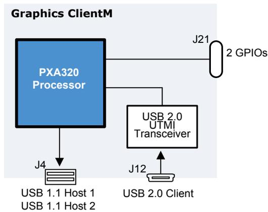
The second option provides a USB 1.1 host port on socket **J4**, a USB 1.1 client port on socket **J12**, and a CSI on socket **J21**. The CSI uses ten of the twelve GPIOs. In this option, only two GPIOs are available for application use on socket **J21**.
