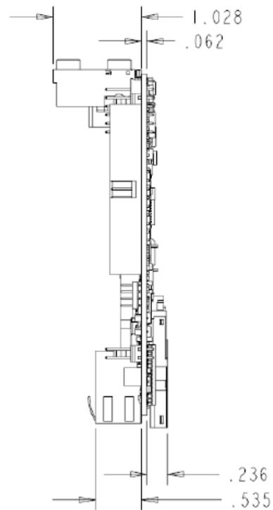
The final view illustrates the underside. Notice socket J2 is located on the underside.
